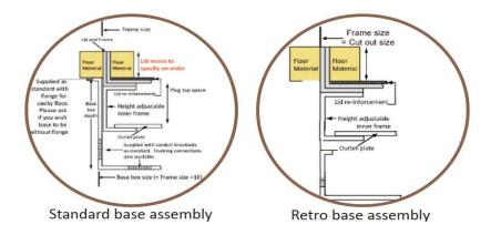
In any case, you would need to know the overall floor depth, the dimensions of the hole in the ground and the exact frame size of the outlet box going in.
